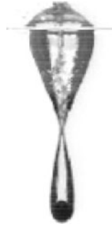
Fig. 3 Cavity due to a high-density sphere ( \rho_p = 2360 \text{ kg/m}^3 ) is cited from Fig. 7 of Duclaux et al. (2007)
